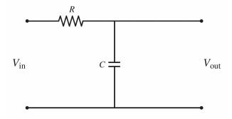
If the input signal  $V_{\rm in} = \sum_{n=0}^{100} V_n \cos(\omega nt)$  is passed through it, where  $\omega = 500$  kHz and  $\{V_n\}_{n=0}^{100}$  are some constants, what would be the resulting output signal  $V_{\rm out}$ .
